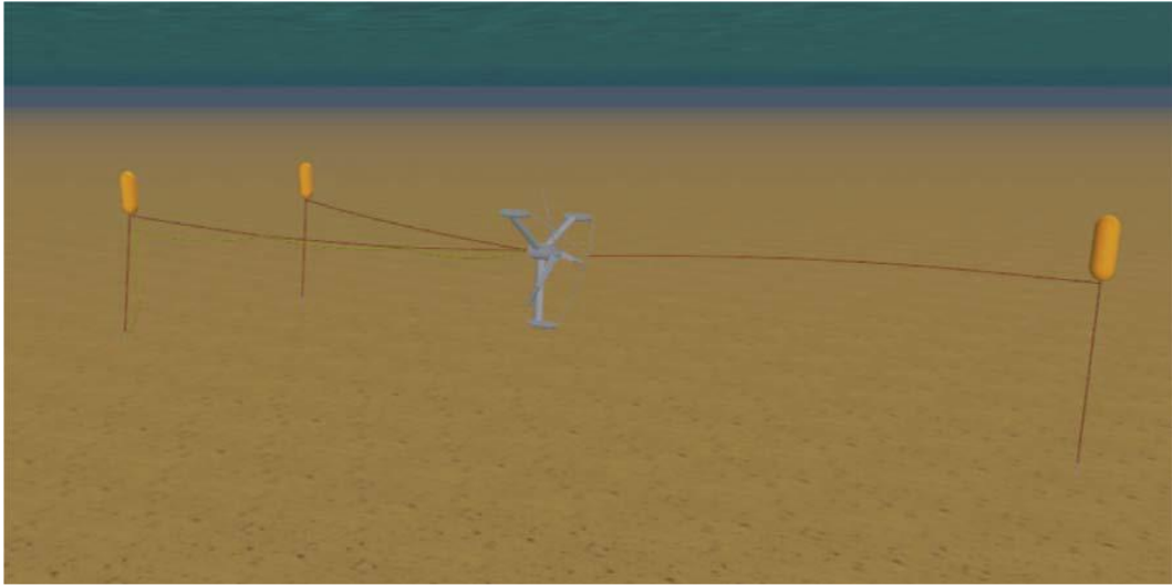
Figure 45: Foundation types: Second generation devices - Mooring system based on wires and buoys.[7]
